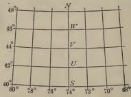
and then six points on the 40° circle are located with the help of the above values of x and y. The distances SU, UV, VW, and WN are next laid off by the help of Table II and through the points thus determined straight lines are drawn
